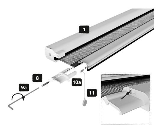
Attach the right grip lock 10b to the side of the guide rail on the roller blind cassette 1. Attach it by screwing in the threaded pin 8 through the hexagonal socket 9a.
