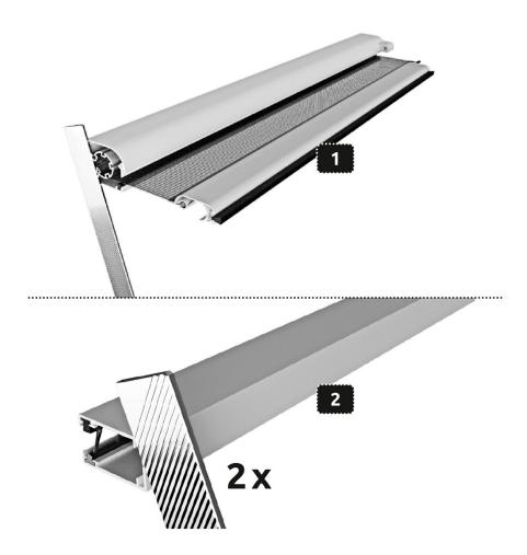
Remove the sealing brush a from the cartridge 1. Pull the sealing brush b from the guide rail and insert it into the downward-facing open groove for later sealing towards the window frame.
