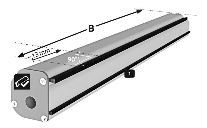
Mark the roller blind cartridge 1 with measurement B minus 13 mm on the side to be shortened. Shorten the roller blind cartridge 1 and grip rail at the marked point with a metal saw. Take note of the position of the cartridge. Example: Measured width of the reveal B = 900 mm - 13 mm = 887 mm. Attention: Risk of injury! Use the saw with caution.
