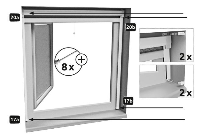
Screw the roller blind above the attachment elements 20a, 20b and 17a, 17b with screws 23. Attach the screw covers 18a, 18b to the top of the roller blind, 21a, 21b to the bottom of the roller blind.
