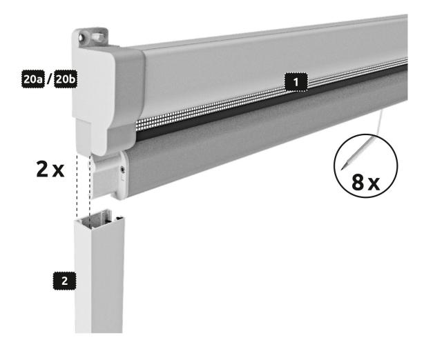
Attach the guide rails 2 via the end caps 20a and 20b to the roller blind cassette 1. Move the roller blind towards the window frame and make a mark of the eight holes through the recesses on the attaching elements 20a, 20b and 17a, 17b. Drill into the window frame with a  $\emptyset$  2,5 mm drill.
