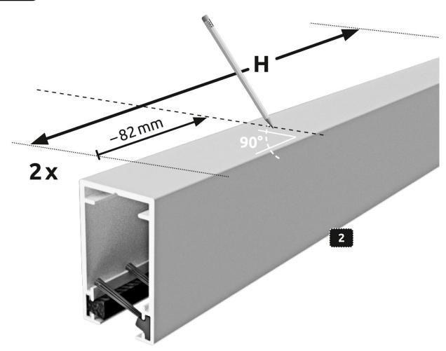
Mark the guide rail 2 with measurement H minus 82 mm. Shorten both guide rails 2 at the marked point with a metal saw. Example: Measured height of the reveal H = 1200 mm - 82 mm = 1118 mm. Attention: Risk of injury! Use the saw with caution.
