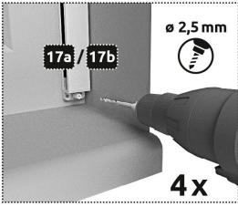
Screw the roller blind above the attachment elements 20a, 20b and 17a, 17b with screws 23. Attach the screw covers 18a, 18b to the top of the roller blind, 21a, 21b to the bottom of the roller blind.
