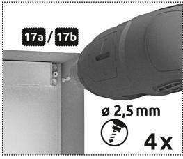
Screw the roller blind above the attachment elements 20a, 20b and 17a, 17b via screws 23. Attach the screw covers 18a, 18b and 21a, 21b to the the roller blind.
