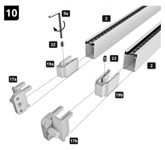
Attach the guide rails 2 via the end caps 20a and 20b to the roller blind cassette 1. Move the roller blind towards the door frame and make a mark of the eight holes through the recesses on the attaching elements 20a, 20b and 17a, 17b. Drill into the door frame with a  $\emptyset$  2,5 mm drill.
