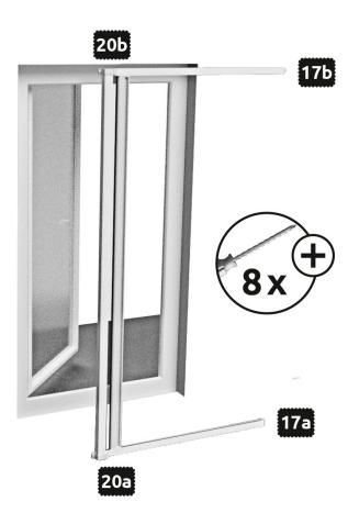
Screw the roller blind above the attachment elements 20a, 20b and 17a, 17b via screws 23. Attach the screw covers 18a, 18b and 21a, 21b to the the roller blind.
