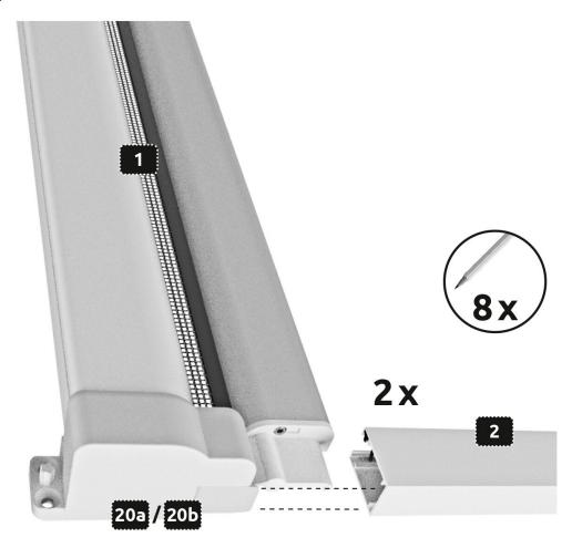
Attach the guide rails 2 via the end caps 20a and 20b to the roller blind cassette 1. Move the roller blind towards the door frame and make a mark of the eight holes through the recesses on the attaching elements 20a, 20b and 17a, 17b. Drill into the door frame with a  $\emptyset$  2,5 mm drill.
