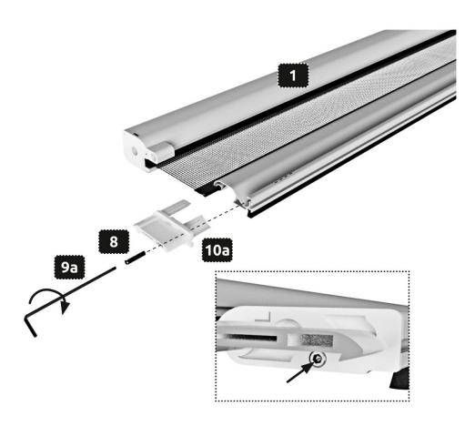
Attach the right grip lock 10b to the side of the guide rail of the roller blind cartridge 1. Attach it by screwing in the threaded pin 8 via the hexagonal socket 9a.
