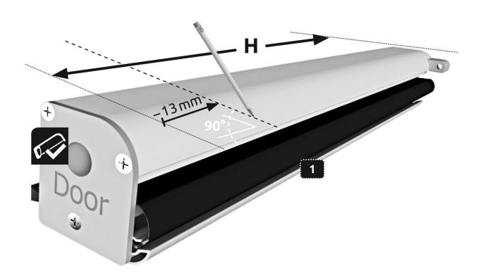
Mark the roller blind cartridge 1 with measurement H minus 13 mm on the side to be shortened. Shorten the roller blind cartridge 1 and grip rail at the marked point with a metal saw. Take note of the position of the cartridge. Example: Measured height of the reveal H = 2000 mm - 13 mm = 1987 mm. Attention: Risk of injury! Use the saw with caution.
