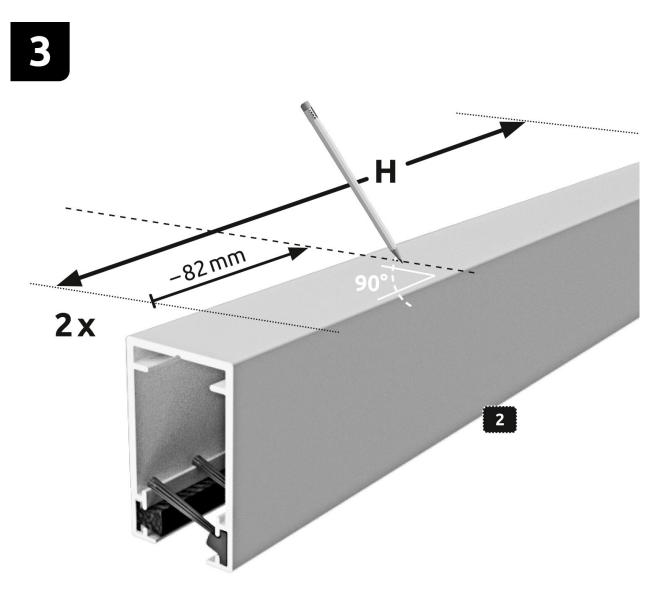
Mark the guide rail 2 with measurement H minus 82 mm. Shorten both guide rails 2 at the marked point with a metal saw. Example: Measured height of the reveal H = 1200 mm - 82 mm = 1118 mm. Attention: Risk of injury! Use the saw with caution.
