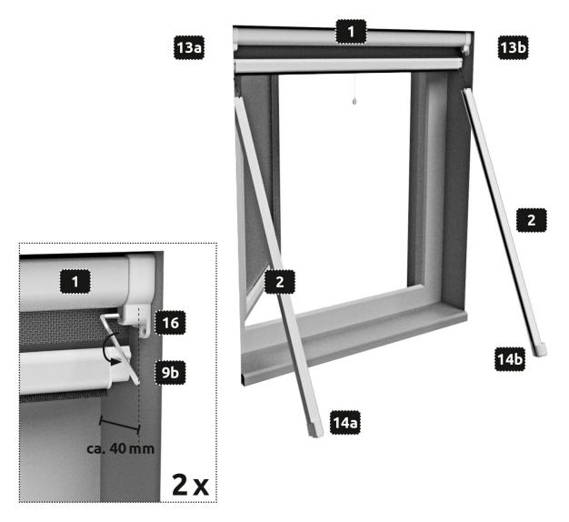
Initially, loosely clamp the roller blind cassette 1 with approx. 40 mm distance to the window into the reveal by using the inner screws 16 via the hexagonal socket 9b. The screw section should point outwards, when doing this. Attach the guide rails 2 via the end caps 13a and 13b with the roller blind cassette 1.
