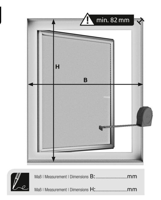
Mark the roller blind cartridge 1 with measurement B minus 13 mm on the side to be shortened. Shorten the roller blind cartridge 1 and grip rail at the marked point with a metal saw. Take note of the position of the cartridge. Example: Measured width of the reveal B = 900 mm - 13 mm = 887 mm. Attention: Risk of injury! Use the saw with caution.
