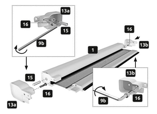
Attach one screw each 16 through the hexagonal socket 9b in the intended middle recess of the end caps 12a and 12b. Connect the lower and upper clamp parts 12a and 14a, as well as 12b and 14b together. Insert the connected clamp units into the guide rails 2. Take note of the position of the depicted individual parts.
