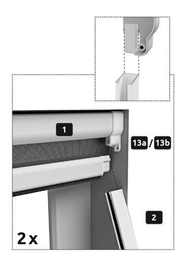
Attach the roller blind through adjusting the inner screws 16 on the roller blind cassette 1 and guide rails 2 via the hexagonal socket 9b in the wall reveal.
