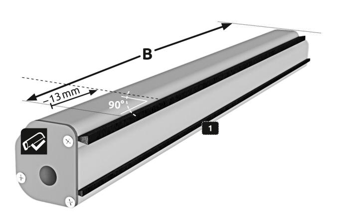
Mark the roller blind cartridge 1 with measurement B minus 13 mm on the side to be shortened. Shorten the roller blind cartridge 1 and grip rail at the marked point with a metal saw. Take note of the position of the cartridge. Example: Measured width of the reveal B = 900 mm - 13 mm = 887 mm. Attention: Risk of injury! Use the saw with caution.
